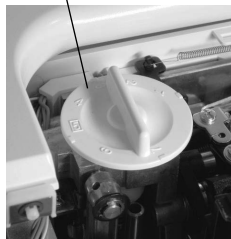
Presser foot pressure adjusting dial
